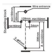
3. Fix the hanging board to two holes which are at the top by using the plugs and screws.
